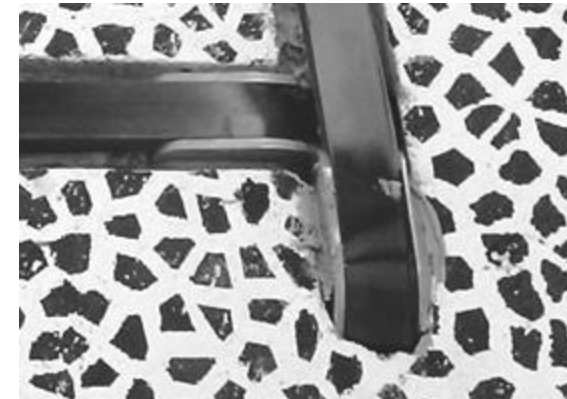
deviators on top surface
